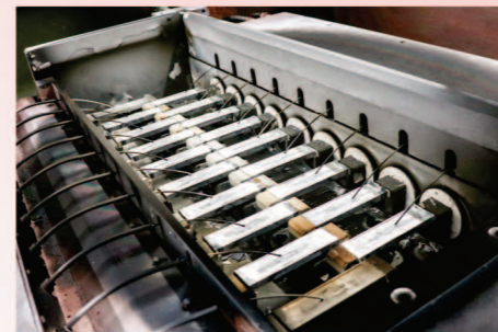
Double Evaporation Sources For Heavy Deposition
